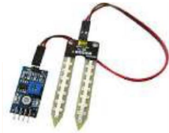
Figure 2: soil moisture sensor
