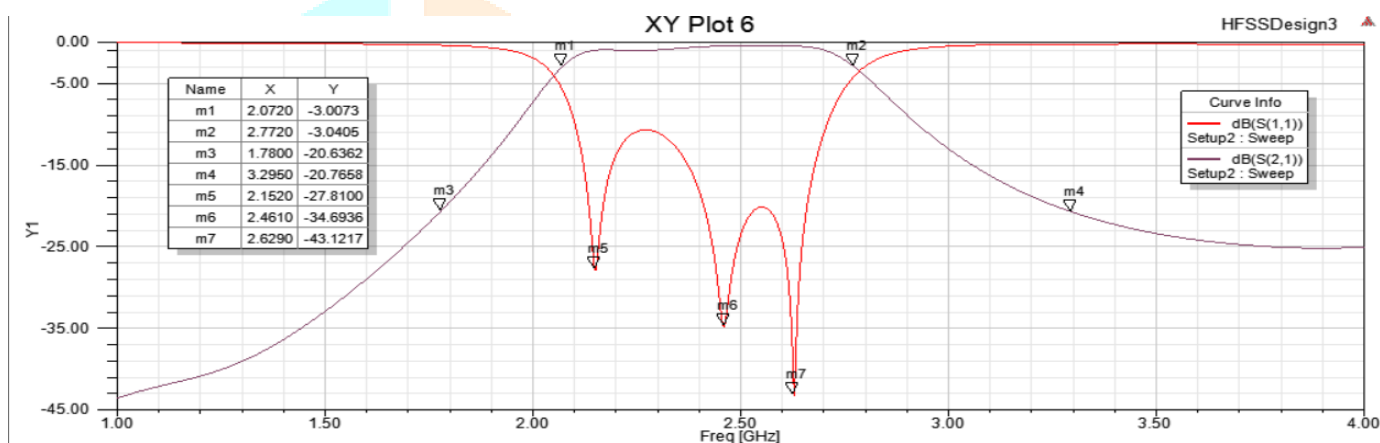
Fig5: Insertion loss and Return loss graph of proposed filter with DGS
