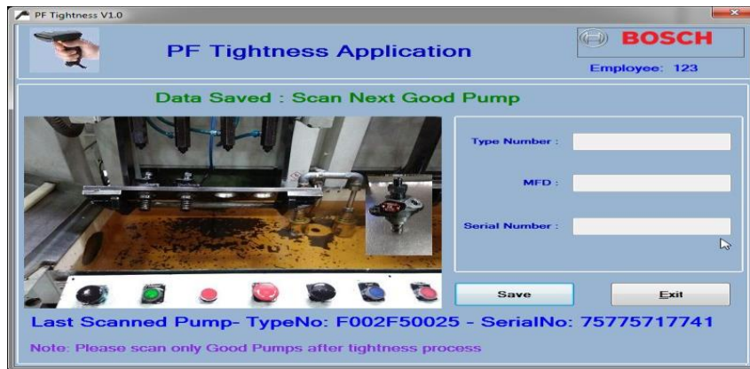
Fig.7: snap shot for scanning the next set of pumps
