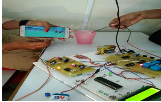
Fig-7.6: Elephant Chase Away Pressure sensor measures the force per unit area of the elephants when they walked so that the movement of elephants is detected. An automatic signal is sent to the sprinkler by the sensor, which sprays the capsaicin on elephants which irritates them and prevents them from entering the field.
