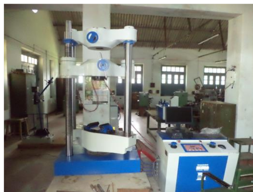
Figure 6: Computerized universal testing machine used in tensile test
