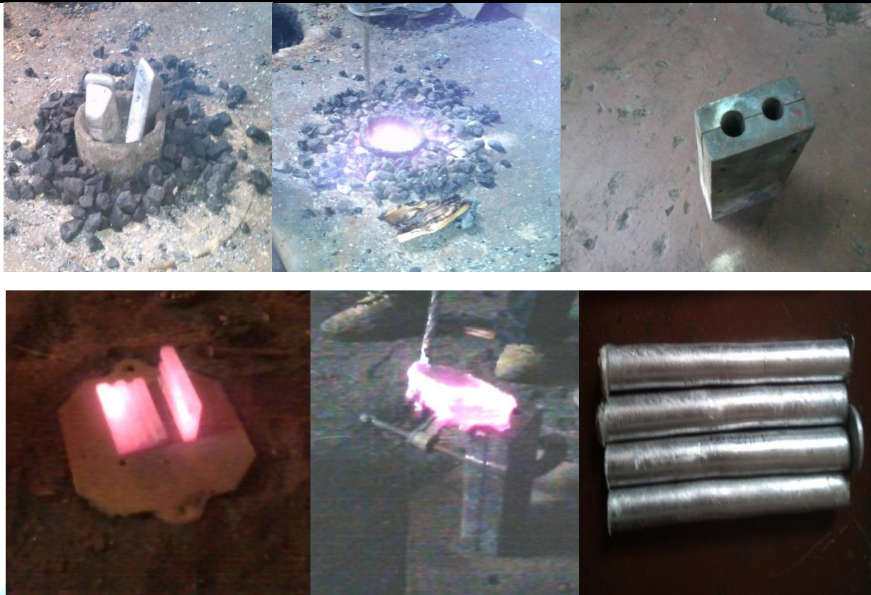
Fig 2: stages in casting: (A) crucible in furnace containing ZA27 ingots, (B) Molten metal in crucible, (C) Cast iron die in cold condition, (D) preheated Cast iron die, (E) pouring of molten MMC in to die, (F) ZA27/SiCp final castings, (G) degassing tablets (hexa-chloromethane)
