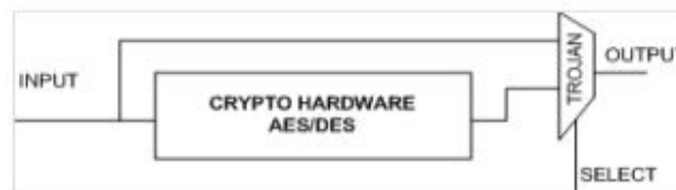
Fig. 2 Basic Block Diagram of Hardware Trojan
