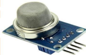
Fig-4: Smoke Sensor
