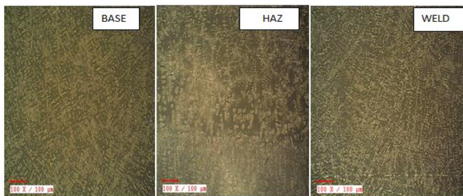
(a) Base Zone (b) Heat affected zone (c) Welded zone Fig.12: Microstructure observation of Aluminium welded sample
