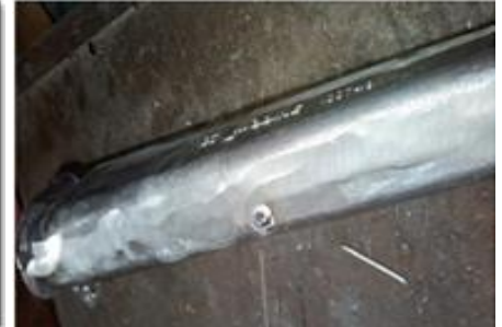
Fig.4: Defected component after welding
