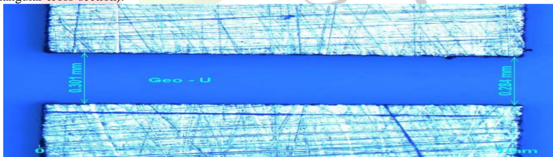
Figure 2.1 Throttle geometry “U” in 300 µm thick sheet steel
