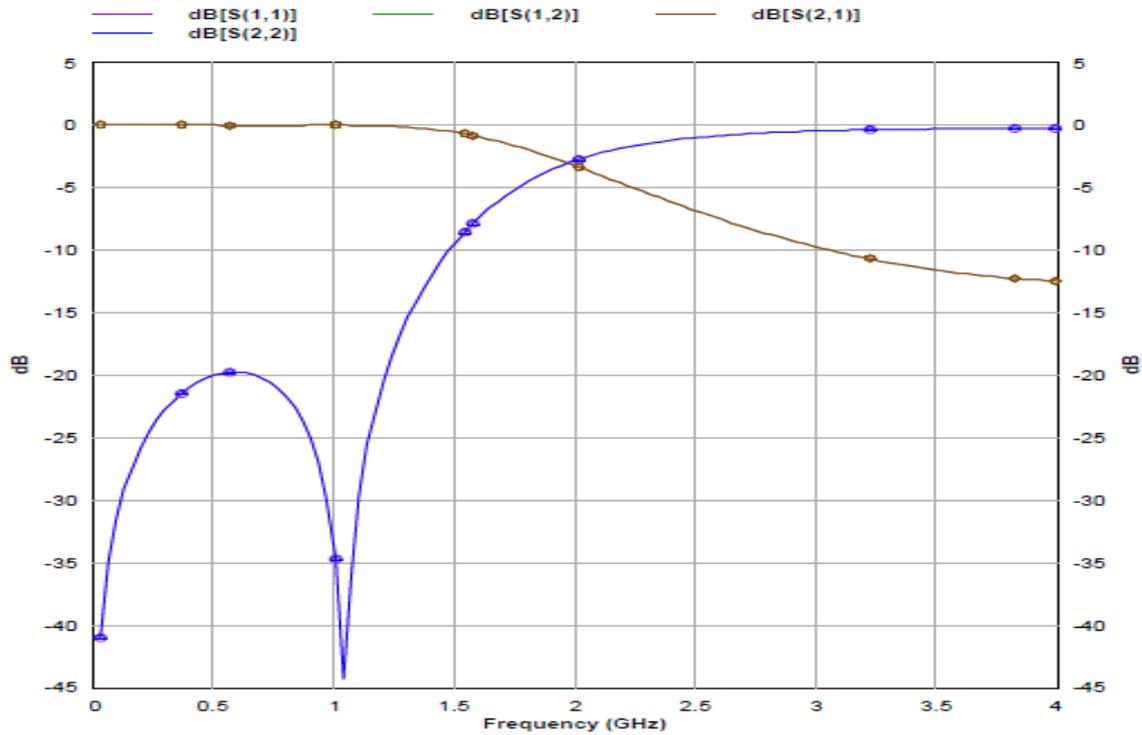
Figure 4: full-wave em simulated performance of third order stepped impedance low pass filter
