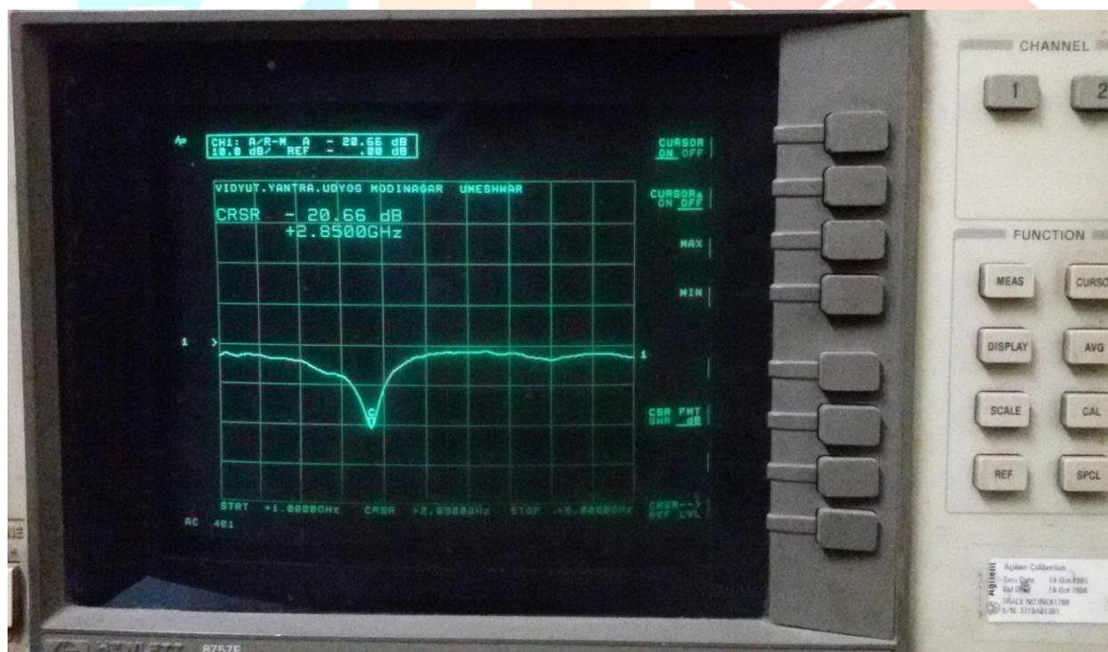
Figure 7: Response of third order stepped impedance micro-strip low pass filter (return loss) using network analyzer.
