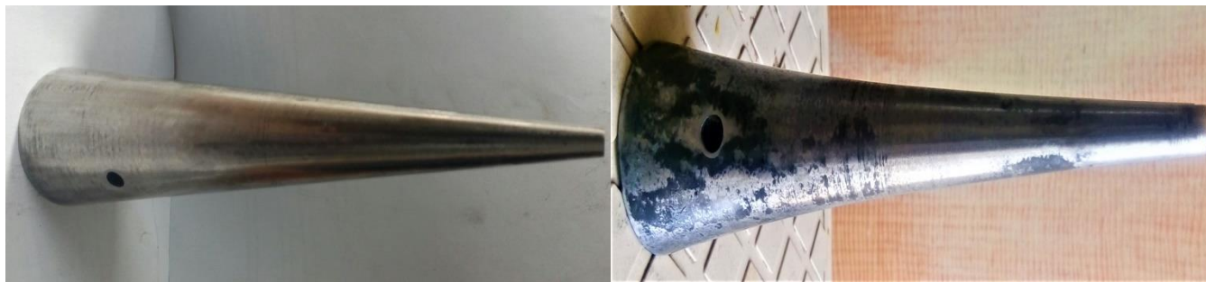
Fig 3.2 Fabricated Conical Sonotrode and Exponential Sonotrode
