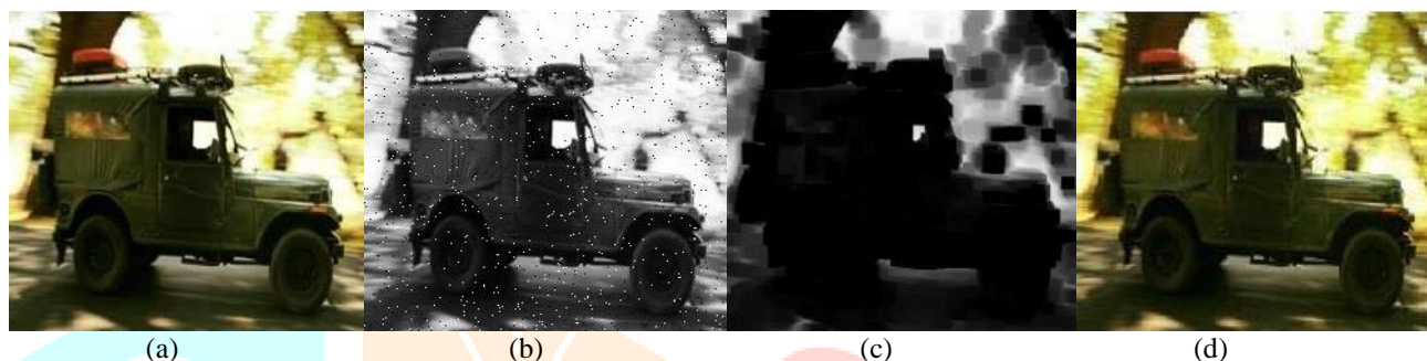
Figure 5(Image 2): (a)Input Degraded Image (b) Salt & Pepper noise (c) Dark Channel Estimation (d) Output Image
