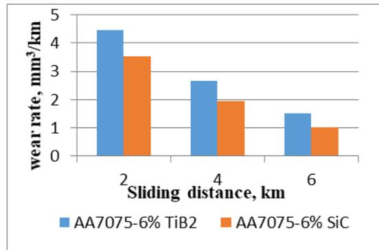
Figure 3.3 Wear Test
