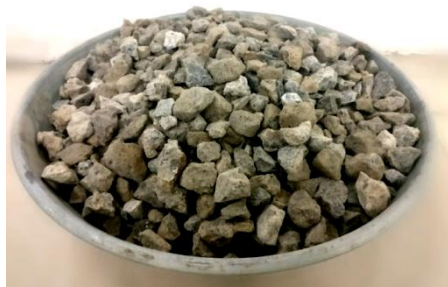
Fig 2.1: Manually crushed recycled aggregates
