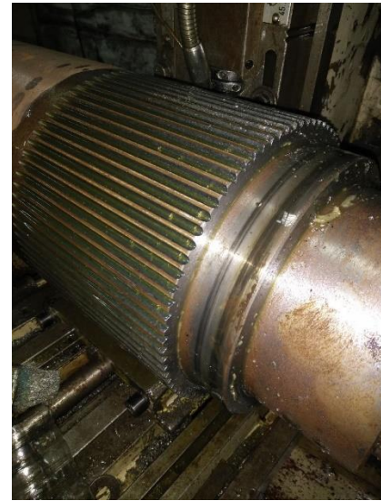
Fig. 9. Hobbing of corrugation roller uniformly over circumference in process
