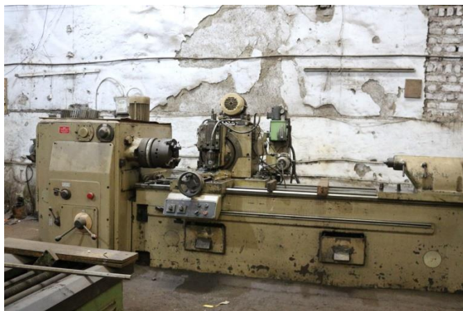
Fig. 8. Semi-automatic long length hobbing machine Make: WMW
