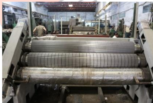
Fig. 3. Rollers fitted on a Fingerless Corrugation Machine
