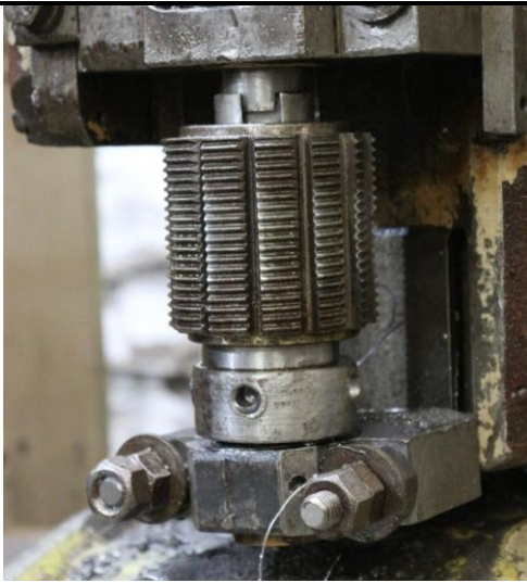
Fig. 6. A Hobbing Tool mounted on a machine
