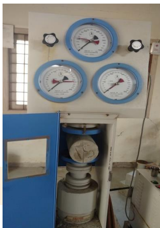
Split tensile test of a cylinder
