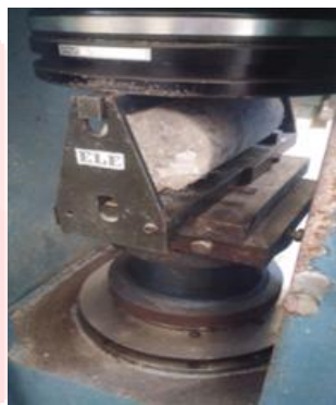
Fig 5: Split Tensile Testing Of Cylinder
