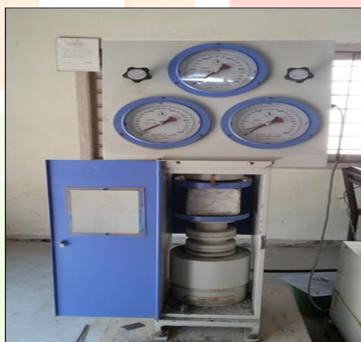
FIG. 1 COMPRESSIVE TEST ON CONVENTIONAL CONCRETE
