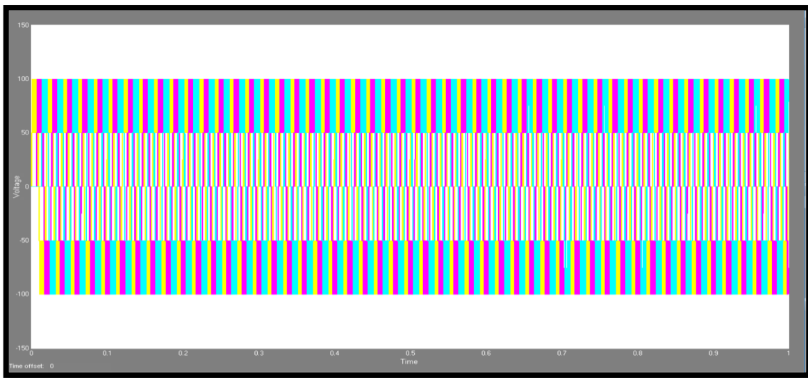
Fig 5.10- Inverter controlled output
