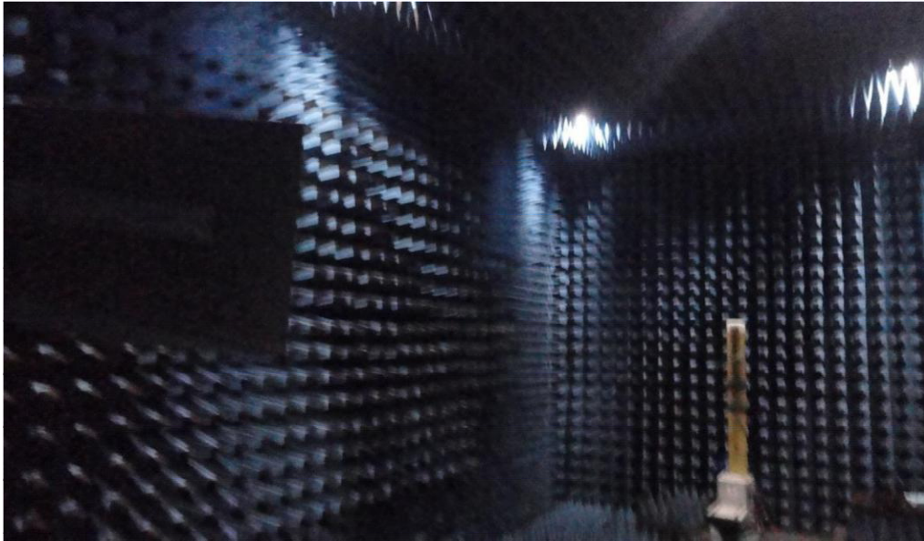
Figure 11 Measurement of radiation pattern for a slotted Octagonal shaped antenna in an anechoic chamber
