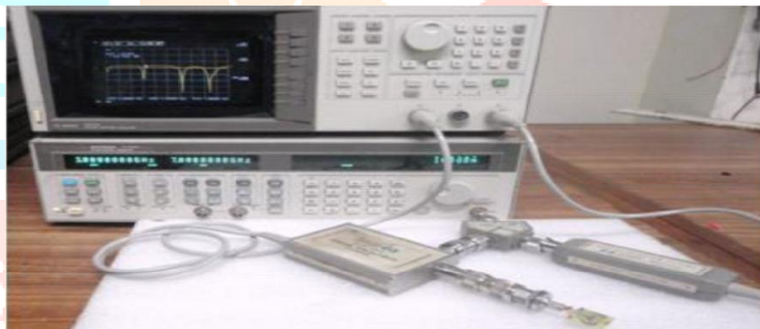
Figure 7 Return loss measurement using HP 8757D Scalar Network Analyzer for a slotted Octagonal shaped antenna
