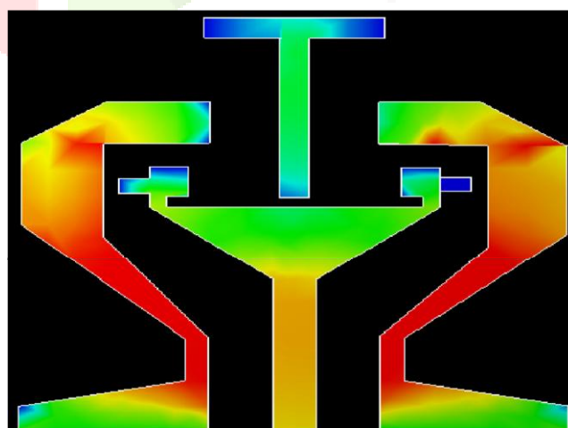
Figure 9 (c) Surface Current Distribution at 6.4 GHz
