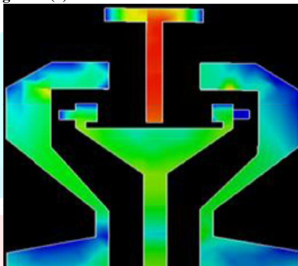
Figure 9 (a) Surface Current Distribution at 4.3 GHz
