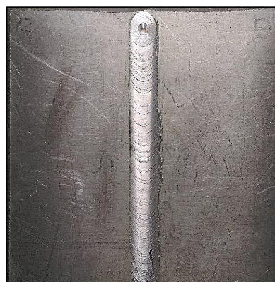
Fig. 3c) Shows the welded plates
