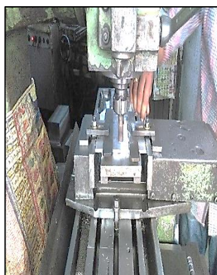
Fig. 3b) Shows the Friction Stir Welding is performed.
