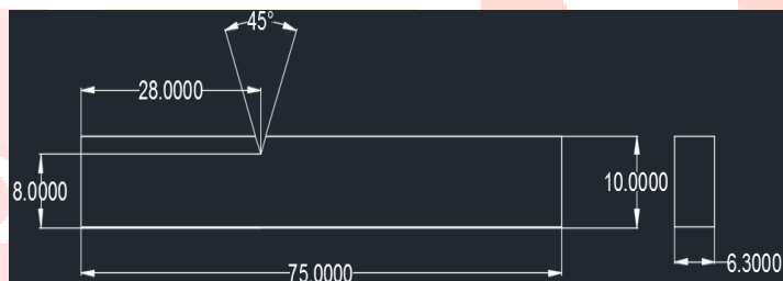
Fig. 5 ASTM E23-16b standard Izod impact test specimen [22]
