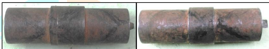
Fig. 2a) Tapered cylindrical pin profile tool
