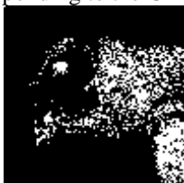
Fig 4.10 Visualization of the NVF image using block averaging of 4X4 non overlapping block The copyright image used in the simulation is shown in figure 411
