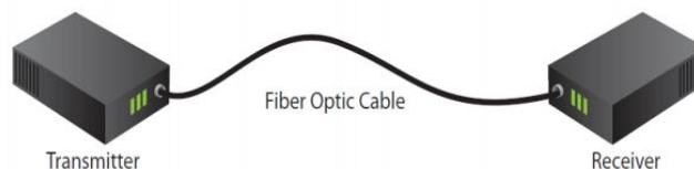
Fig 1.1: Basic Fiber Optic Transmission System
