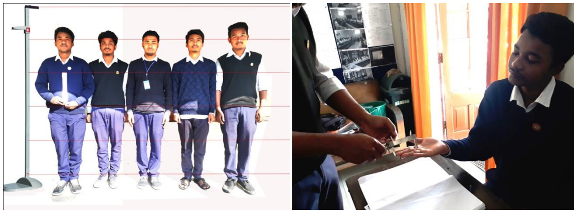
Fig. 1: Measurement of Stature and figure length using Stadiometer and vernier calipers.
