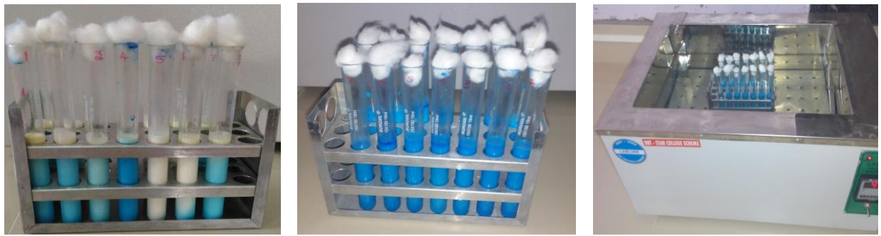
Image 1, 2 and 3: Incubation and decolourisation of samples inside the water bath (42±1 0 C)
