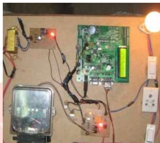
Fig 6. Wireless meter reading system PCB when the load is ON and the interfacing of Energy meter, ARM7 (LPC 2148) Microcontroller modules.
