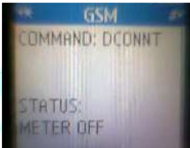
Fig.9: By sending the command “#DCONNT” through the mobile phone the GSM modem receives the command and the load will be disconnected and an reply message will be sent to the mobile phone regarding the current status of the system.
