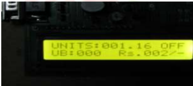
Fig.10: LCD showing the power consumption values and the billed amount and status of the system is also displayed when it is OFF.
