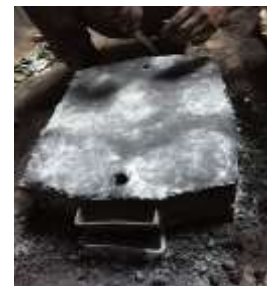
Fig.5 – sand casting mould
