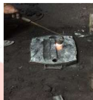
Fig.6 – Sand heating for fixed the sand properly
