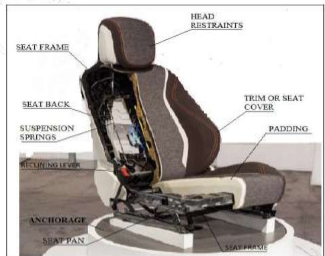
Fig-1: Cut section of driver seat components and systems
