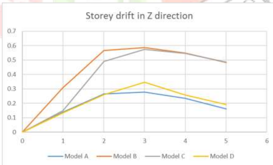
Fig. 5.2: storey drift in z direction
