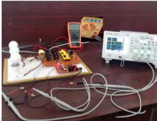
Fig. 14. Experimental setup of a slide mode control dc-dc interleaved boost converter
