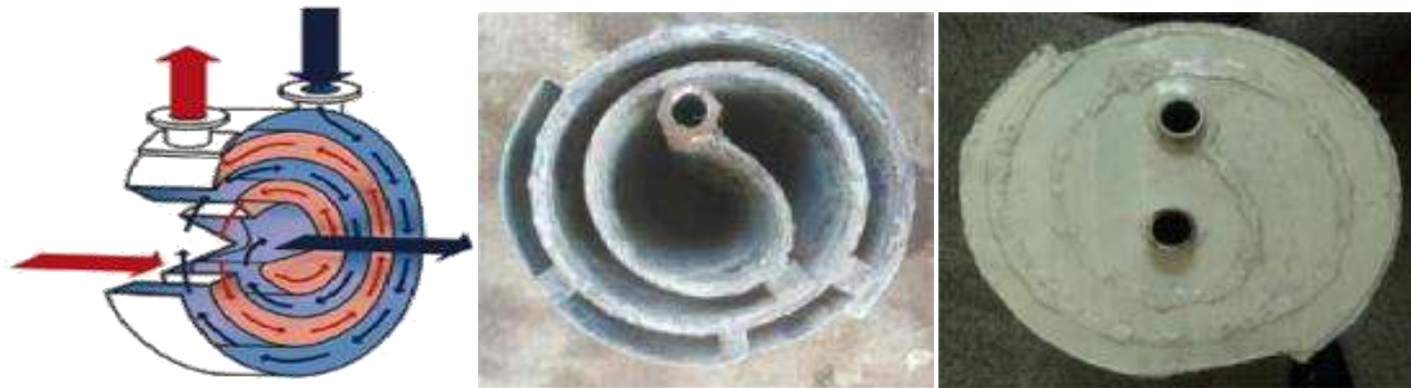
Fig.9 (A) Spiral plate heat exchanger (B) Hot and cold channels (C) Completed heat exchanger
