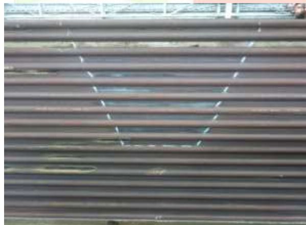
Fig.5. Marking of Distortion
