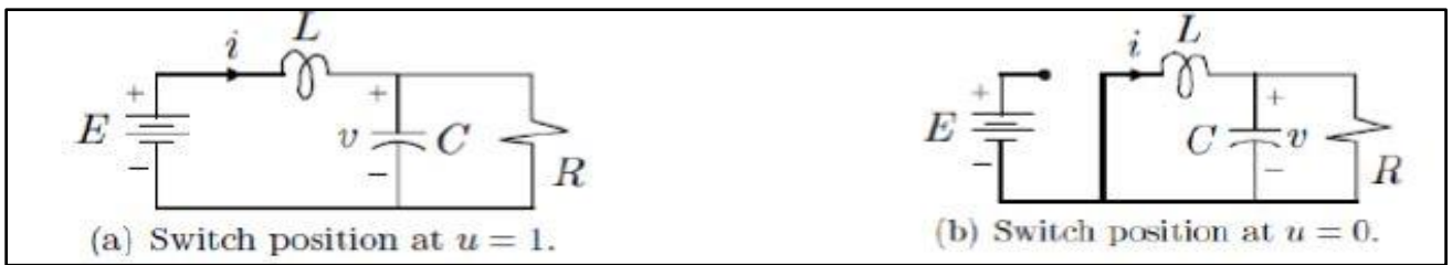
Fig2: Operation mode of a DC-DC converter
