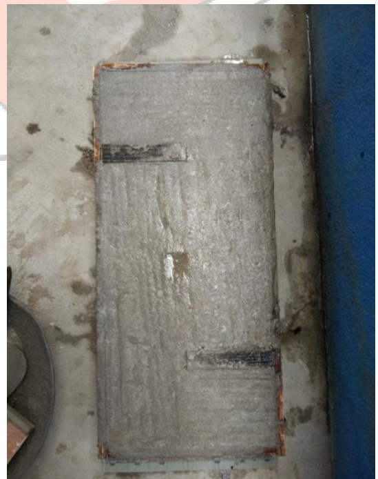
Fig 4 Casting of Push-Off Specimen
