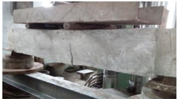
Fig 7 Testing of Beam Specimens
