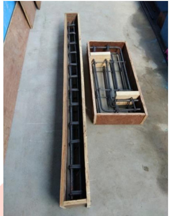
Fig 3 Beam & Shear Moulds With Reinforcement
