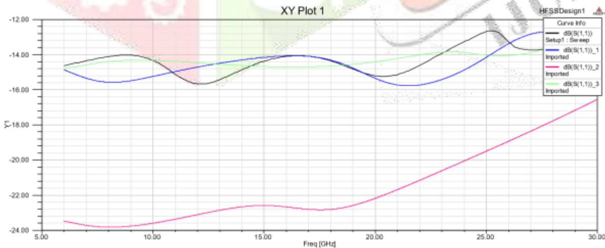
Figure 8: Comparison graph of the stimulated results with different defects in the ground structure
