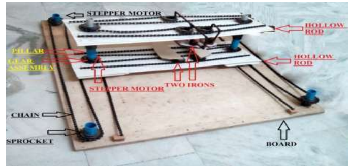
Fig 1.1 Automatic ironing machine based on chain and sprocket mechanism
