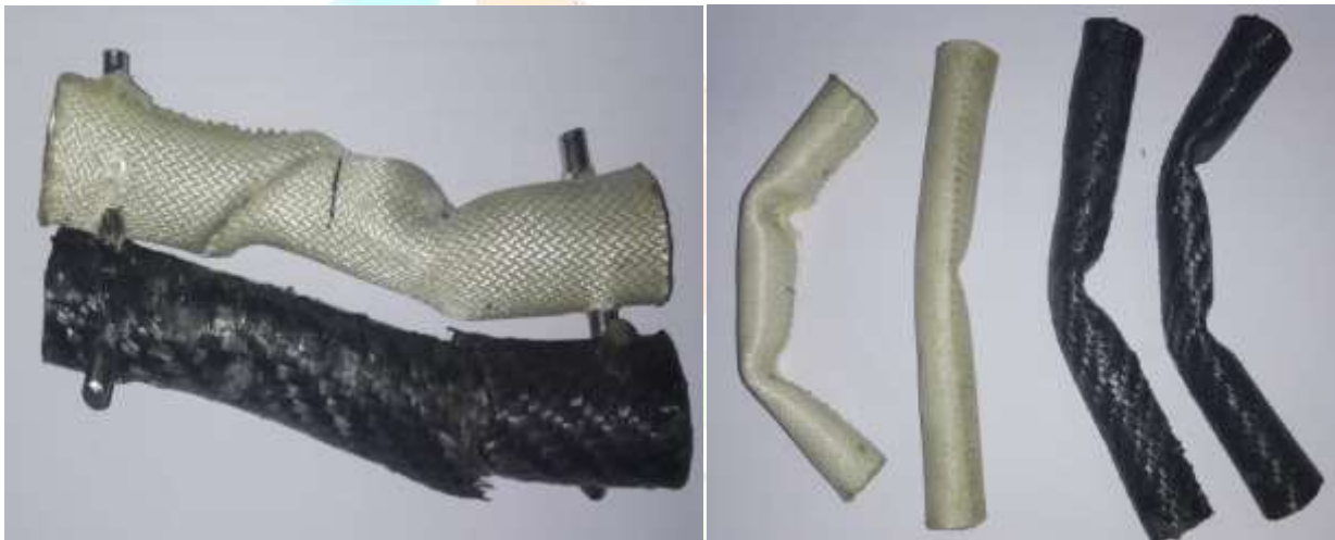
Fig.6: Specimens after torsion and Bending test Respectly
