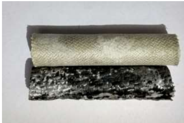
Fig.8: Specimens after NaCl solution
