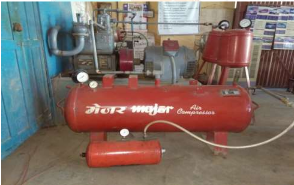
Fig.2: arrangement of compressor unit and pressure cylinder
