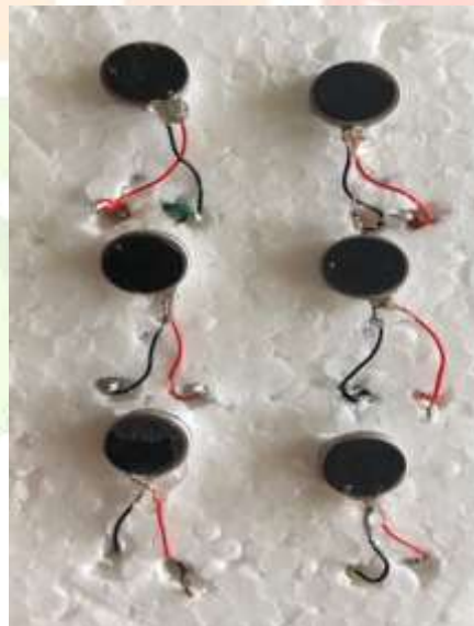
Fig 6.2.3 Vibration Motors arranged in 3*2 matrix format to decipher the characters.
