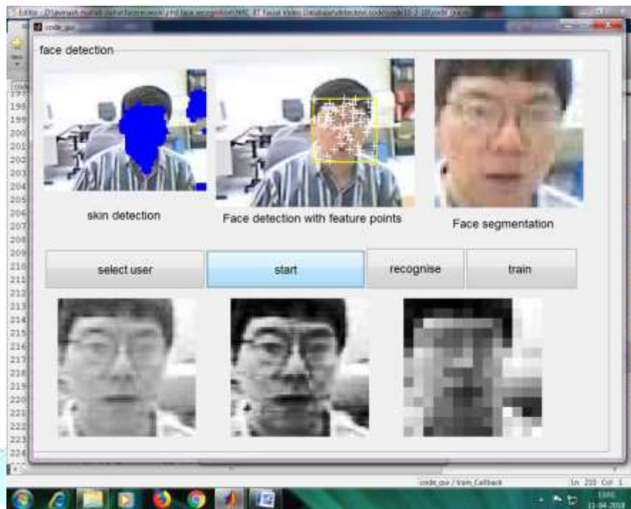
Face 1: Skin detection--face detection—face segmentation—gray conversion—histogram equalization—wavelet decomposition:
