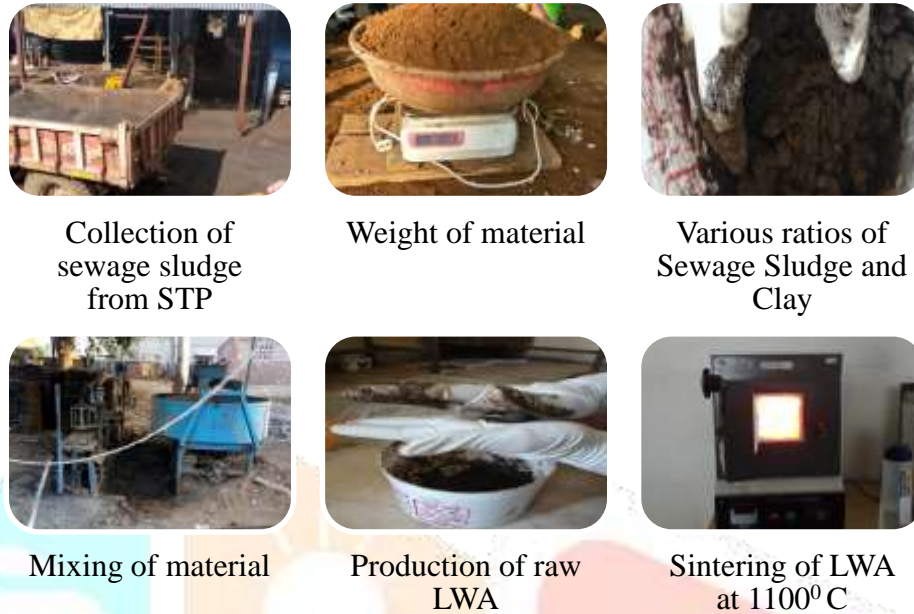
Figure 1 Manufacturing process of lightweight aggregates
