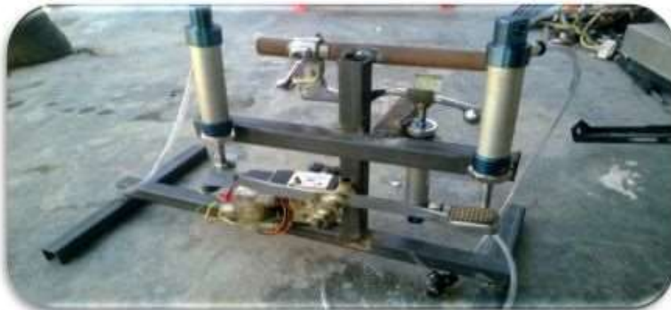
Fig 1.4 Pneumatic, PLC Controlled, Automatic Gear Shift, Vishnu P.R., et.al
