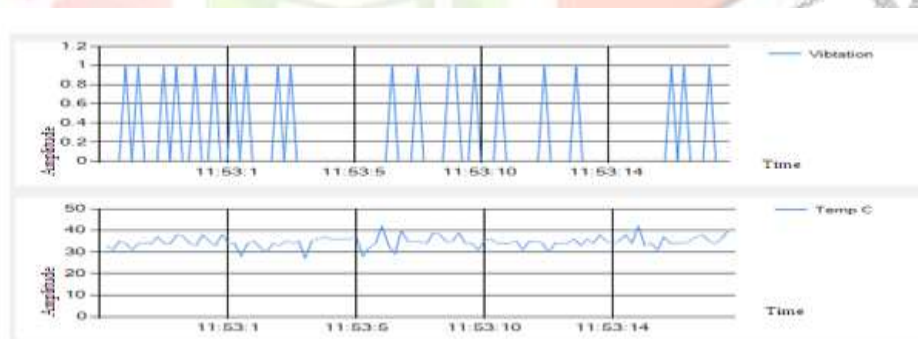
Fig. 7 vibration signal of motor in off condition
