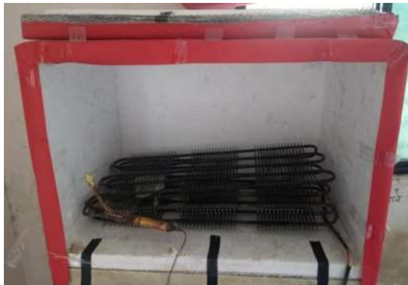
Fig 5 Insulated Box with condensor coils
