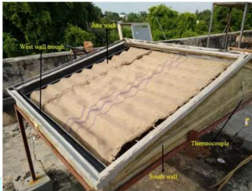
Fig. 18 Photograph of solar still with jute wick [10]
