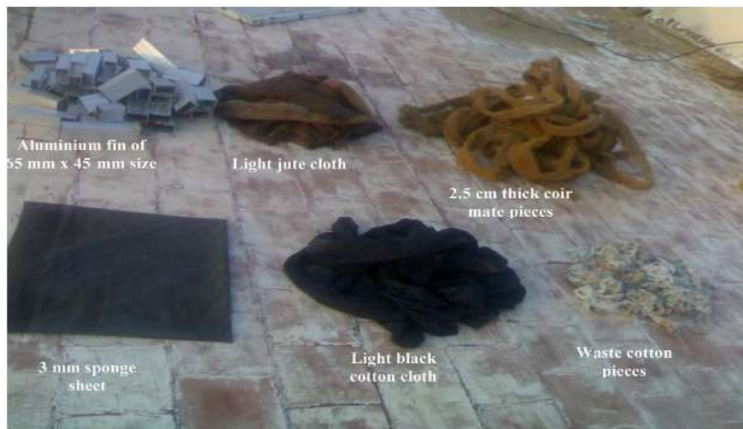
Fig. 10 Different wick materials used in solar still [7]
