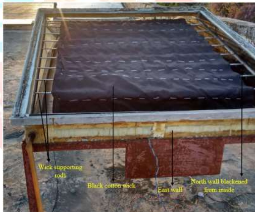
Fig. 19 Photograph of solar still with black cotton wick [10]
