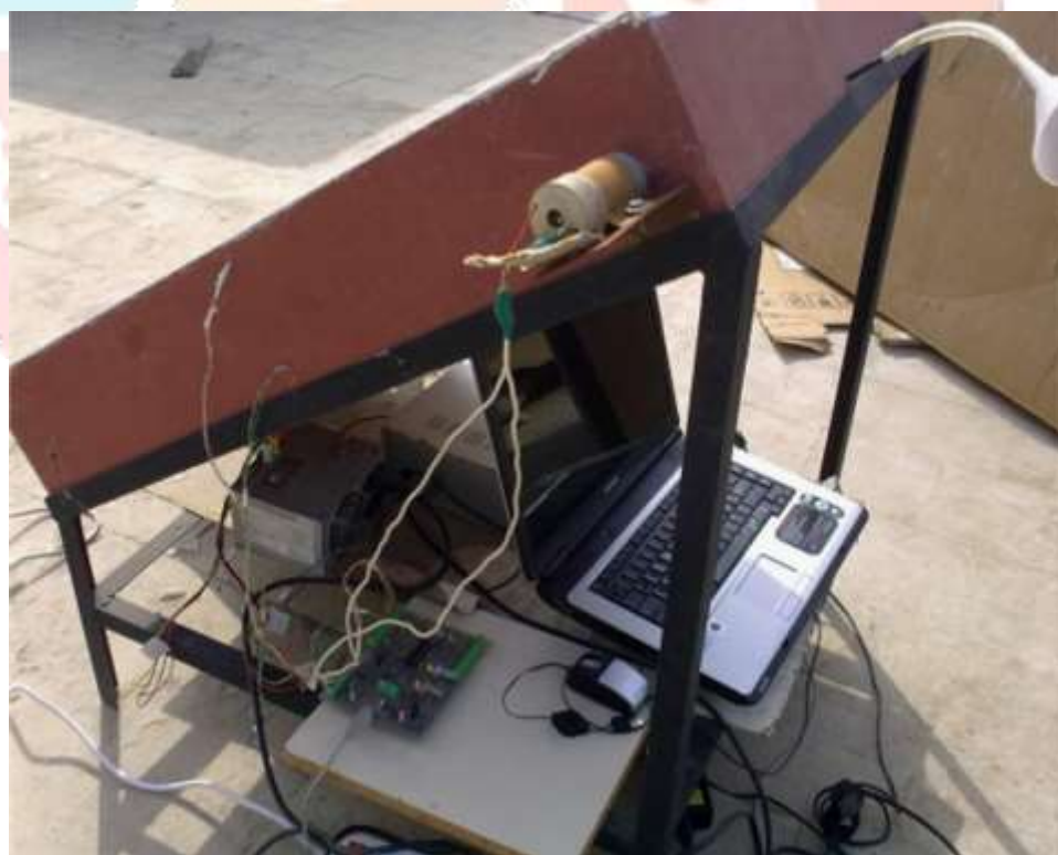
Fig. 22. Experimental setup of solar still having charcoal as thermal energy storage material.
