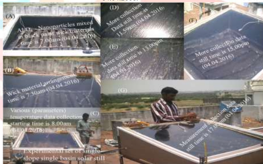
Fig. 11. Photograph of the experimental analysis of single basin still with different fin wick absorbing materials data collection on 04.04.2016.
