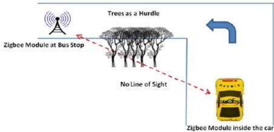
Figure 11. Zigbee Communicate with No Line of Sight (trees as hurdle)
