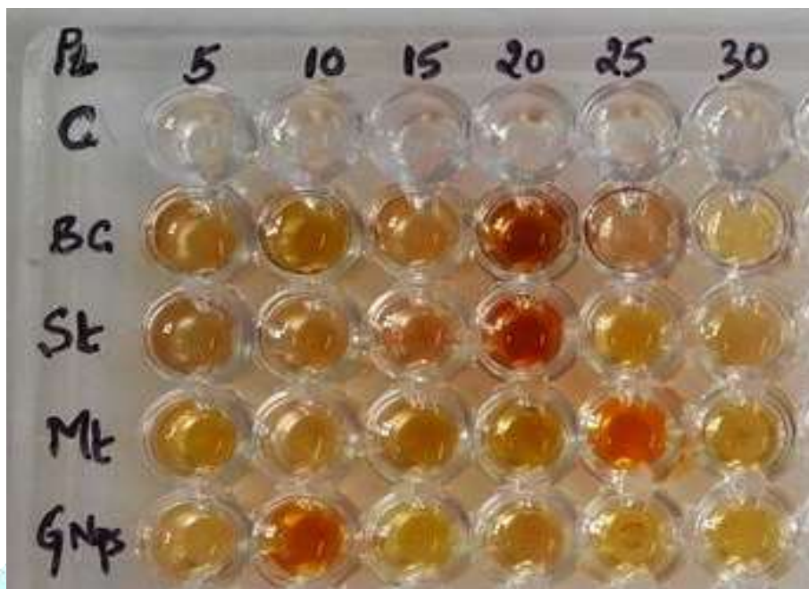
Figure 5 : Change of color intensity over a period for the detection of phenol constituents in the effluent of plastic industry
