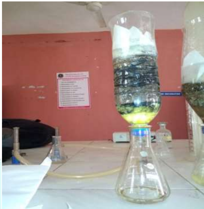
Fig. 4: Filtering with Rice Husk Ash bed
