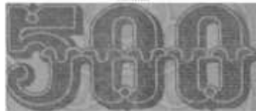
Fig. The gray scale image first eroded then opened by a 5x5 structuring element
