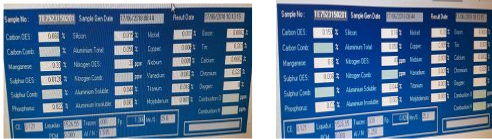
Figure-9 & 10 depicts the different grades mixed during trial of 0.06% C , 0.35% Mn to 0.15 % C & 0.8% Mn and silicon from 0.015 % to 0.16 %.
